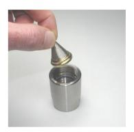
2 | Remove Pos.4 and 5 carefully out of the recess using part no. 101969.
