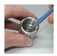
3 | Spray the thread of Pos.1 and Pos.2 with the cleaning agent part no.E99-9.
