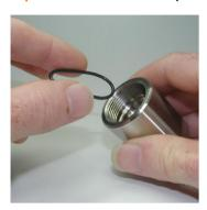
2 | Slightly spread apart Pos.4 and place it into the recess of Pos.1. Take care of installation position!
