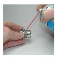
4 | Remove adhesive residues completely from the thread using part no. 63416.
