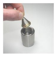
4 | Adhere Pos.2 with Pos.1 using part no. 90160. Apply adhesive all around the first thread of Pos. 2. Screw Pos.2 with Pos.1 using part no. 82284, part no. 61461, part no. 59575, part no. 47475 and part no. 59758, tightening torque **60 Nm**.
