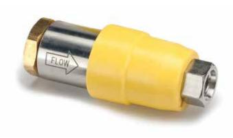
Parker's NGVBCN2-P50 fill line breakaway provides an important safety feature for CNG dispensing systems. It is certified to ANSI/NGV4.4/CSA12.54 standards for breakaway devices used on natural gas dispensing hoses and systems. It allows the hose to safely disconnect, preventing damage to the dispenser in the event of a "drive off" and sealing the CNG in the fill line to effectively prevent leakage or hose whip.
