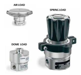
TESCOM 26-2300 Series is a highly accurate, diaphragm sensed backpressure regulator. It controls pressures up to 500 psig / 34.5 bar and offers many  $C_V$ s from 0.02 up to 1.0. Air and dome loaded versions are available for remote operation or for use with the TESCOM ER3000 Electropneumatic Controller for automation.
